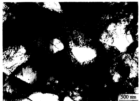
Fig. 1. TEM bright field image of Mo–1.0wt%TiC at low magnification.
